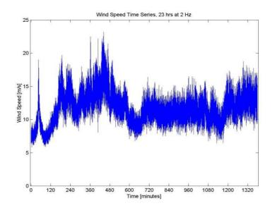
Figure AA.3: Typical wind data, sampled at 2 Hz for a 23-hr period
