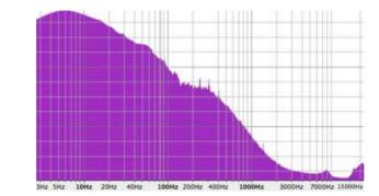
Figure AD.3: Frequency content of typical wind turbine measurement. (from Palmer ASA paper.)
