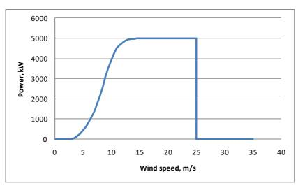
Figure AA.8: Typical wind turbine power curve
