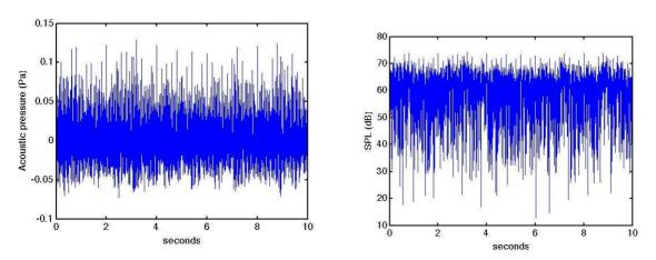
Figure AD.2: Pressure signal from a wind turbine
