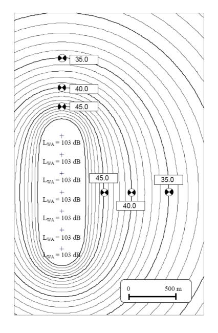
Figure AE.2: Sound pressure level due to a line of seven wind turbines, each operating at a sound power level of 103 dB(A) (from Materialien 63
