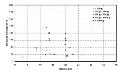
As may be seen in the figure, the maximum distance that ice was observed to fall from a turbine with a diameter of 20 m during operation was approximately 100 m. Based on the observed data, Seifert et al. suggest the following simplified formula for the maximum throwing distance:
