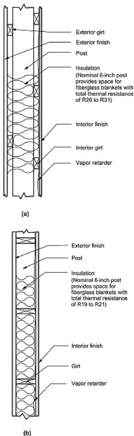
**Figure 2** Typical post frame wall sections with (a) girts on exterior and interior of posts, and (b) girts between posts.
