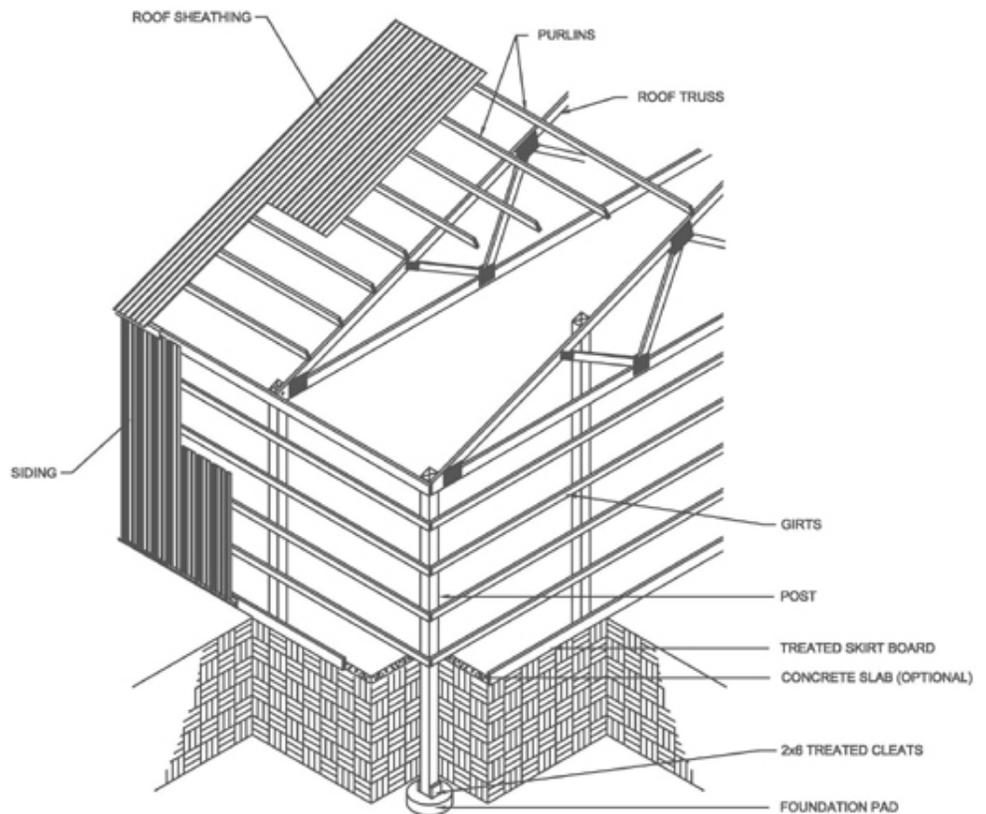
**Figure 1 Components of a Post Frame Building**
