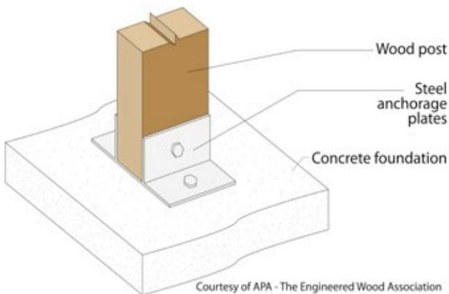
**Figure 4 Post anchorage (post pinned) typical for glued-laminated columns**
